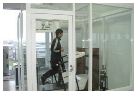
Environment simulator room in which the oxygen concentration can be controlled
