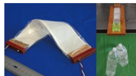
Figure 2) High-power and light-weight electrostatic artificial muscle
